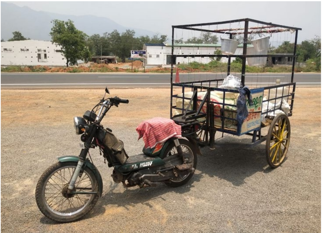
Figure 5.3: Indian 'Jugaad' turns TVS XL sport heavy duty moped into a trolley
